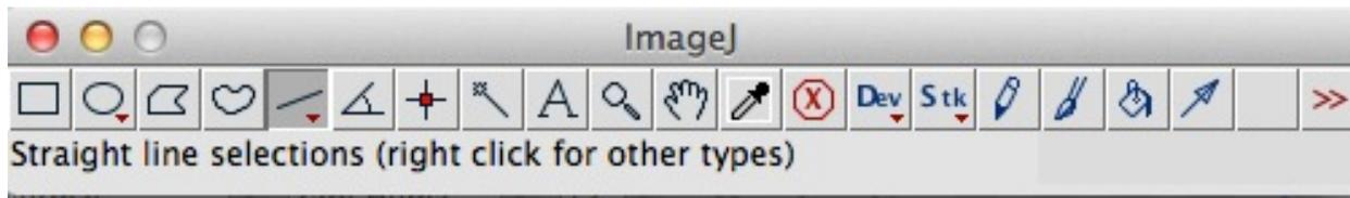
3. Use the **straight line selections tool** to draw a line across the crater's diameter. The length will be displayed under the buttons as you go. Once you let go of the mouse, the measurement will disappear. What is the diameter of the crater in pixels?
